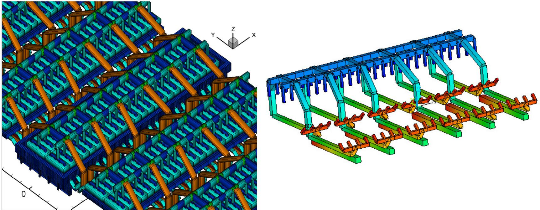
Original RCC busbar network concept with downstream risers
