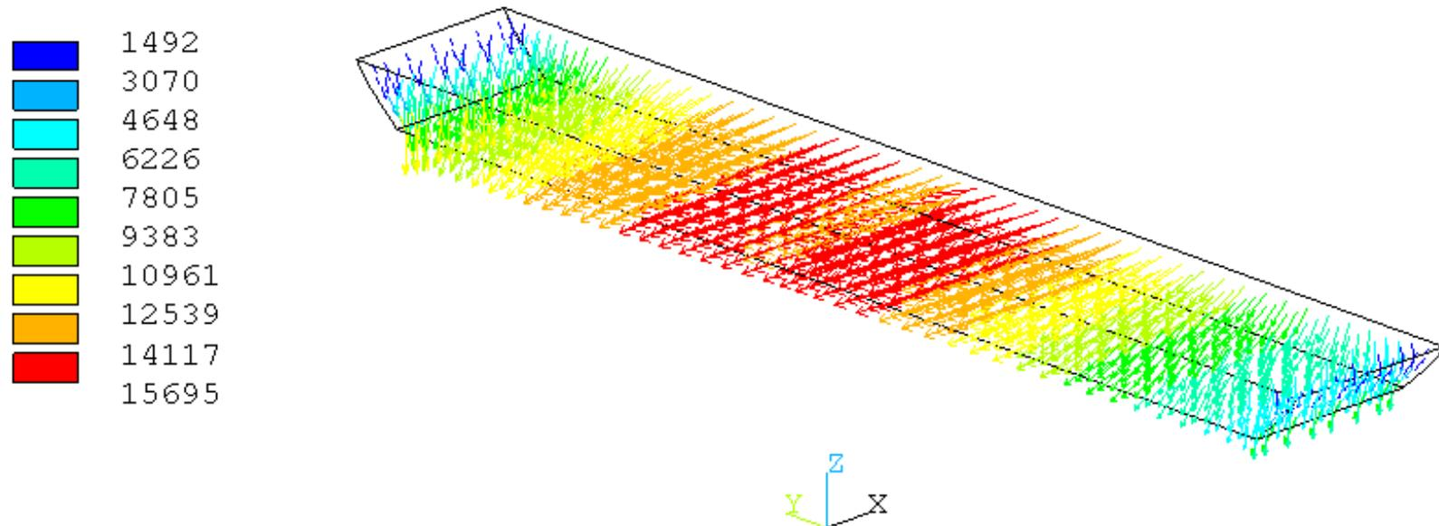
Thermo-electric model metal pad current density
