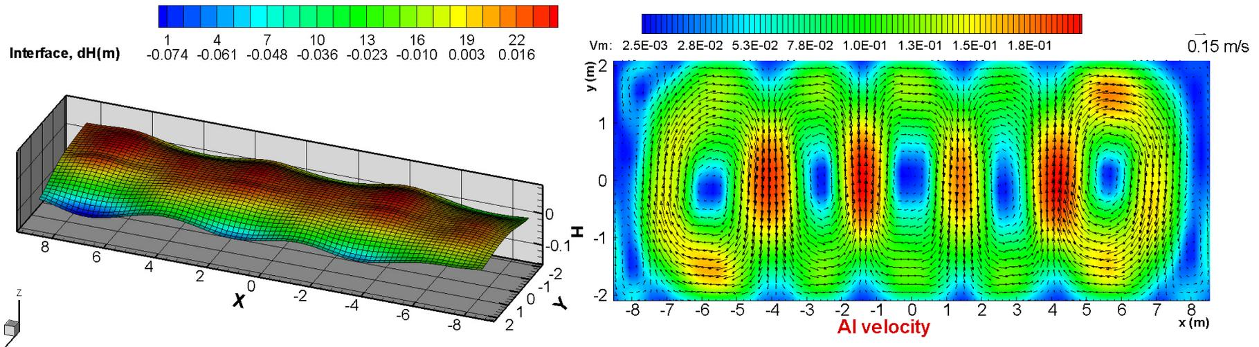
Corresponding steady-state bath-metal interface deformation and steady-state metal pad flow velocity field
