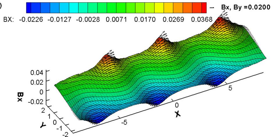
Corresponding  $B_z$  and  $B_x$  magnetic field components
