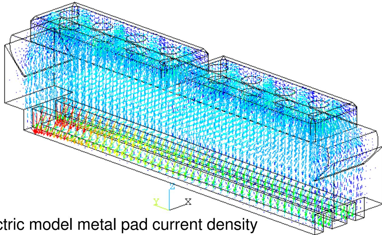
Thermo-electric model metal pad current density
